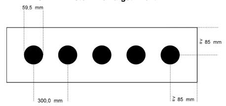
The Diameter of the Black is 59.5 mm with a tolerance of +0.2 mm - 0.0 mm
